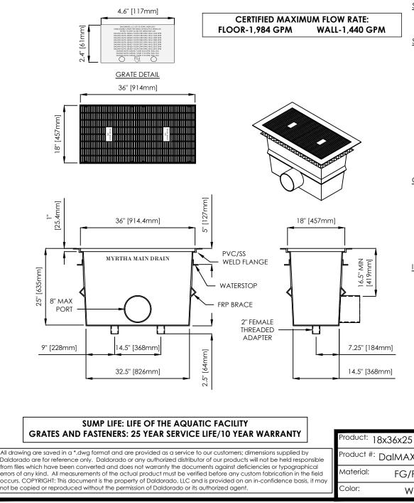
SUMP AND GRATE: UNBLOCKABLE SOFA CERTIFIED TO APSP/ANSI/ICC-16 2017, NSF/ANSI/CAN 50-2020, AND USPC. RPD FIELD CERTIFICATION IS NOT REQUIRED.
